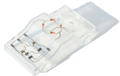
LBS sintered LED Circuit. Ag on PC
